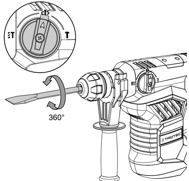
4. Turn the function selector switch (3) back to the **T** position to continue working.
