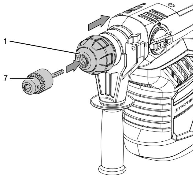
3. Then release the SDS-plus system tool holder (1).
