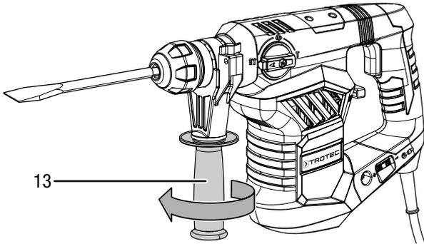
2. Turn the additional handle (13) into the desired position.
