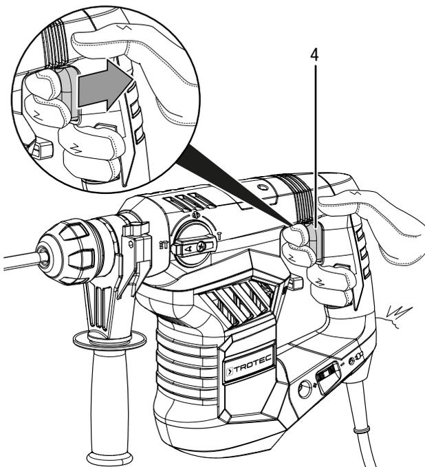
7. Let go of the on/off switch (4) to stop the device.
