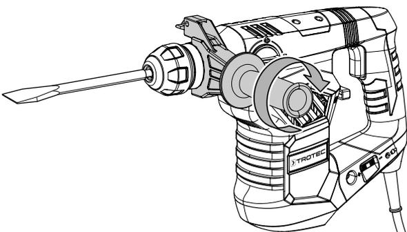
4. Check the additional handle (13) for tight fit. If necessary, tighten the additional handle further.
