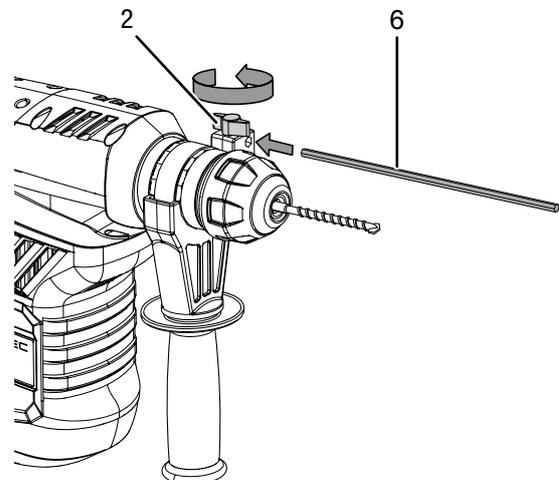
3. Adjust the depth stop (6) to the desired length.
