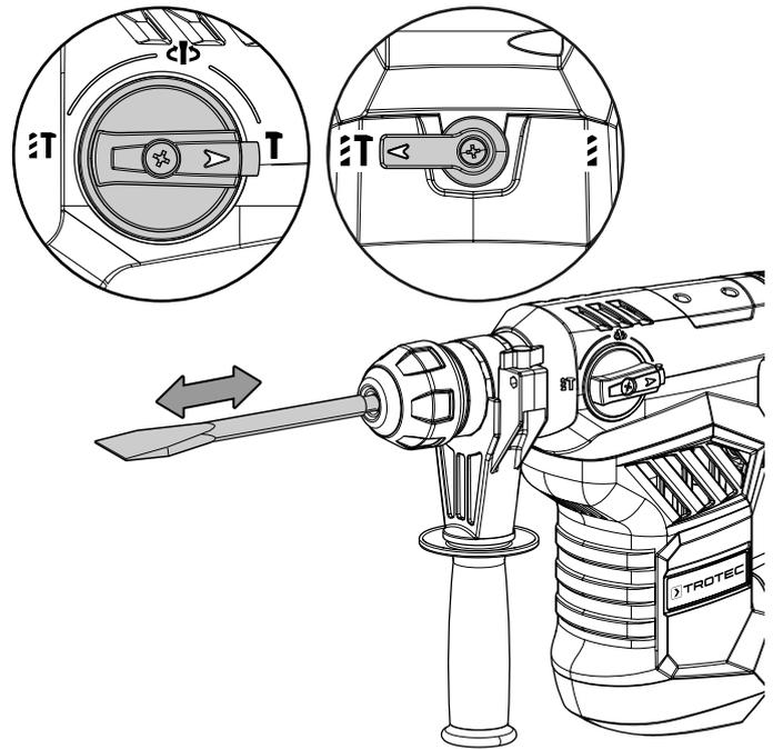
⇒ Operating mode: Hammer drilling
