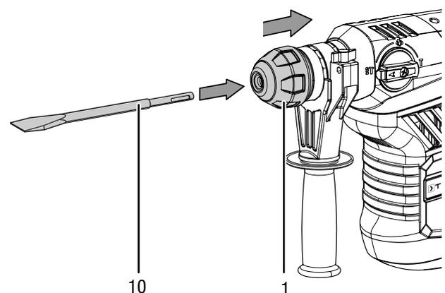
3. Then release the SDS-plus system tool holder (1).
