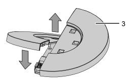
2. Turn the two catches (5) at the bottom side of the foot by about 90° to lock the two foot parts together.
