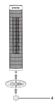
3. Tighten the plastic nut (4) at the bottom side of the fan body.
