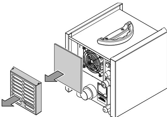
2. Clean the filter using a slightly damp, soft, lint-free cloth. If the filter is heavily contaminated, clean it with warm water mixed with a neutral cleaning agent.
