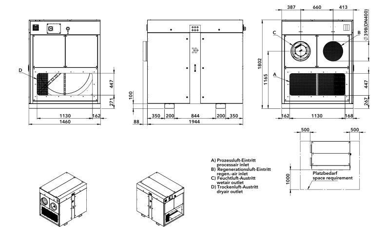
Subject to change without notice. All performance data refer to 1013 mbar, a density of 1.2 kg/m³ and a power supply with 3x400 V/50Hz +PE or 230V/50 Hz. For your project design we recommend to consider a safety discount of 10-20 % for the dehumidification performance depending on the application.
