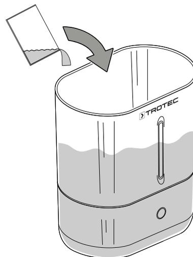
3. Insert the SecoSan® Stick (optional accessory) (12) into the water tank (6).
